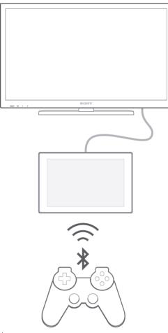
To set up a connection between a DUALSHOCK™3 wireless controller and your device, a USB On-The-Go adapter is required.
